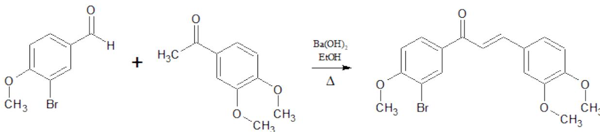
**Figure 1.** Reaction of 3-bromo-4-methoxybenzaldehyde, 3,4-dimethoxyacetophenone, and barium hydroxide to produce a chalcone analogue
